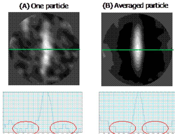
**Fig. 3. Images of one particle (A) and averaged particle (B). The averaged image is generated from 63 images of iron oxide particle. The corresponding line profiles are shown below the particle images.**
