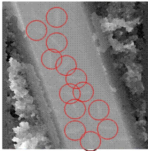
**Fig. 2. Electrostatic phase image of spindle-shaped iron oxide particles. The phase image is obtained from electron holography technique. Circles indicate each particle which is picked up for particle classification.**
