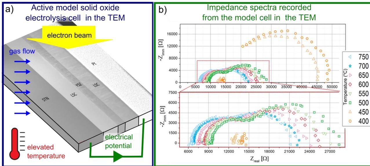
Fig. 1: (a) TEM image of the model SOEC with drawings added to illustrate the cell geometry and the in situ conditions: gas flow, elevated temperature and electrical potential. (b) Impedance spectra recorded from the model cell in (a) during exposure of  $\text{O}_2$  at 400-750°C.
