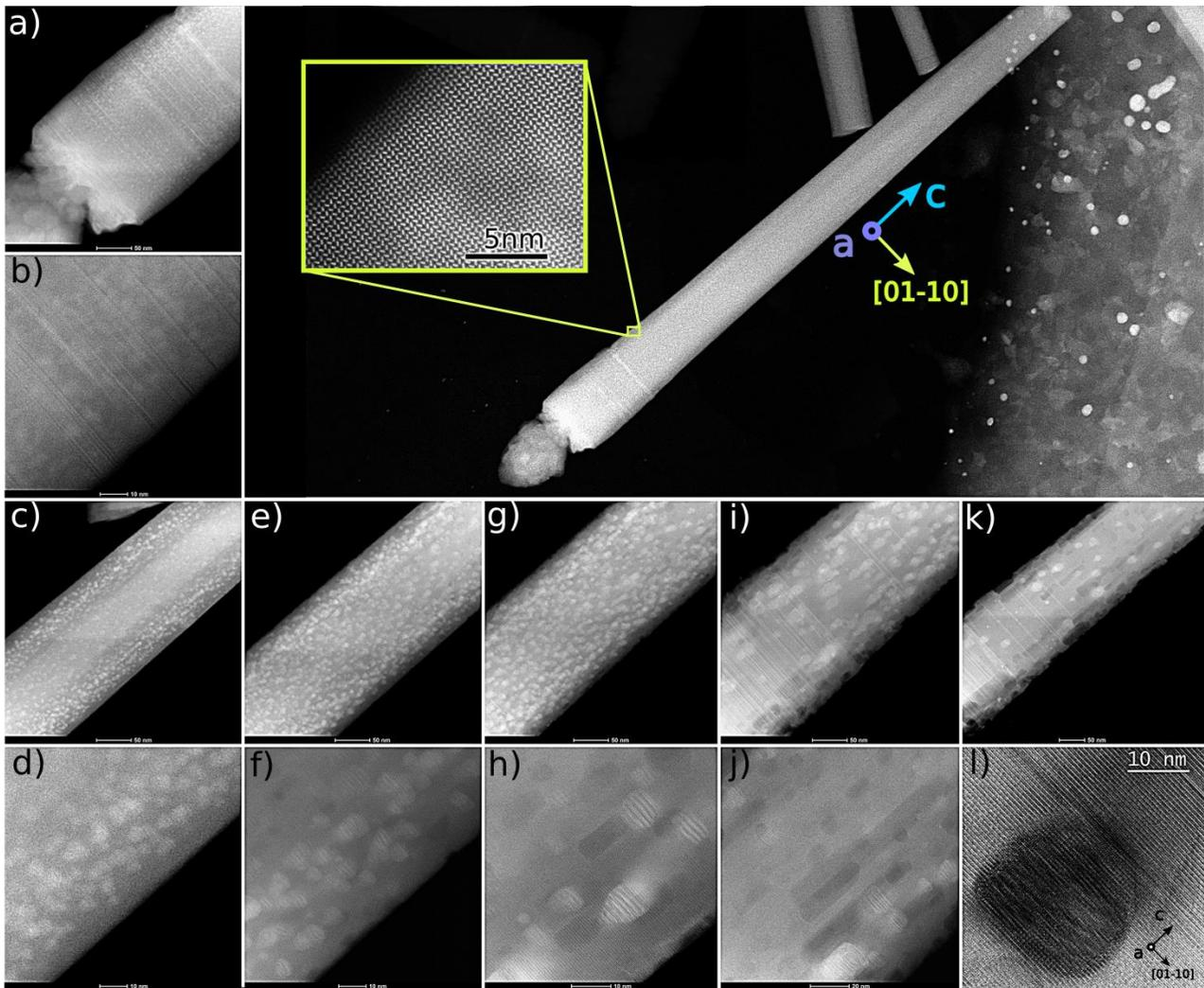
**Fig. 2** Scanning Transmission Electron Microscopy (STEM) images of the typical as-grown WZ NW (left top) placed on the heating chip and its structural changes while in-situ annealing measurements in: **a,b)** 350°C **c,d)** 400°C **e,f)** 450 °C **g,h)** 500°C **i,j)** 550°C **k)** over 600°C **l)** HRTEM image of one MnAs nanoprecipitate. Annealing was performed in double tilt heating holder and phase transformation was observed in perfect zone-axis.
