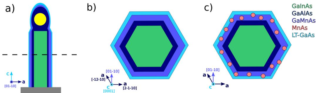
**Fig. 1** **a)** Schematic model of core-shell NW grown in MBE. Cross-sections cut along dashed line of: **b)** as grown NW, **c)** post-annealed NW with visible precipitations.
