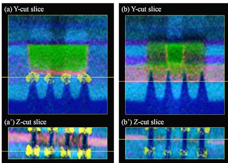
Figure 1 Y and Z slice maps from the elemental map reconstructed by EDS tomography. The Z-cut slice is parallel to the wafer surface. Positions of the Y-cut and X-cut slices are indicated by yellow lines shown in the corresponding Y and Z slice maps. The germanium in the stressor, the tungsten in the electrode and the silicon in the channel and substrate are colored yellow, green and blue, respectively.
