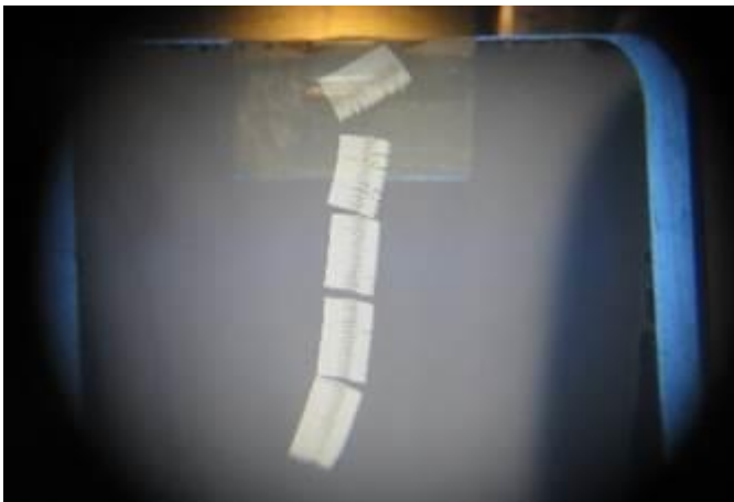
Fig. 1. Ultrathin sections obtained by this protocol. Note five groups of serial sections about 1.8 mm long are already separated after cutting.
