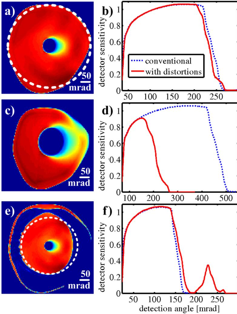
Fig 1: Left: Tilt based detector scans for different camera lengths ((a)196 mm; (c)102 mm; (e)301 mm). The dotted circle shows the expected outer border from the conventional method. The right column shows the resulting radial sensitivities in comparison with conventional curves.
