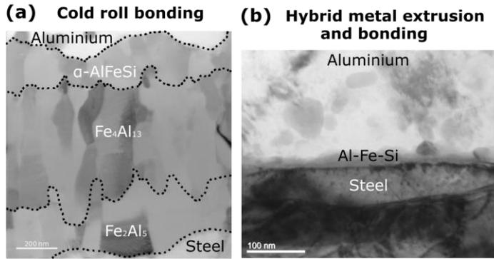
**Figure 1:** (a) Virtual bright field image created from SPED data, that shows the three phases (cubic  $\alpha$ -AlFeSi,  $\text{Fe}_4\text{Al}_{13}$  ( $\theta$ ) and  $\text{Fe}_2\text{Al}_5$  ( $\eta$ )) found at the interface of an aluminium-steel joint made by CRB. The black dashed lines indicate the borders between the different phases. (b) Bright field TEM image of a narrow IMC layer containing aluminium, iron and silicon, found at the interface of an aluminium-steel joint made by HyB.
