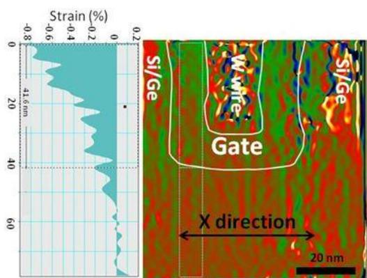
Figure 1. Strain map of a finFET device (right), and line profile of compressive strain  $\epsilon_{xx}$  along a yellow rectangle area in the map (left).
