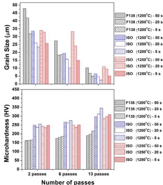
**Figure 3** - Grain size evolution (upper) and microhardness (lower) dependence on the pass number and interpass times for F138 and ISO 5832-9 steels
