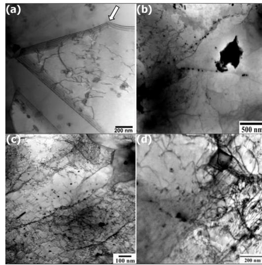
**Figure 2** - Thin foils TEM analysis of ISO 1250oC after 13 passes with 20 or 50 s of interpass time: displaying the interaction of the precipitates with grain boundaries (a) and (b); dislocations (c) and (d).
