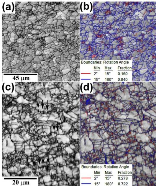
**Figure 1** - EBSD from samples with 13 passes, interpass time of 5 s. (a) and (b) for F138. (c) and (d) for ISO (1200°C) with interruption immediately after the straining. Image quality map: (a) and (c). Orientation Image Mapping (OIM) showing high angle (grains -  $\theta > 15^{\circ}$  - blue lines) and low angle (subgrains -  $2 < \theta < 15^{\circ}$  - red lines) grain boundaries: (b) and (d).
