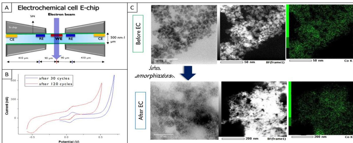
Figure 1. (A) Electrochemical E-chip use in the in situ LP-STEM set-up. (B) Cyclic voltammograms of Co<sub>3</sub>O<sub>4</sub> in OER conditions in situ after 30 cycles and after 120 cycles. (C) Pre and post-mortem STEM images and EDX mapping of the catalysts nanoparticles.
