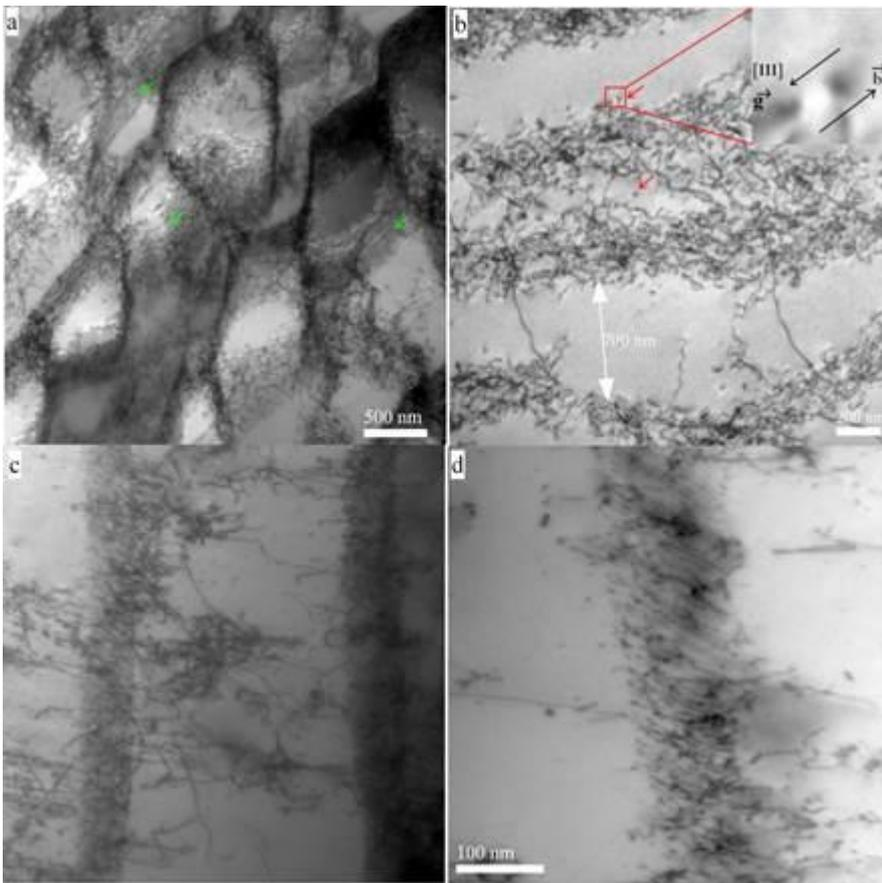
Fig. 2(a-d) Defect structures in SS 316LN subjected to LCF- Creep-HCF interaction at 923K
