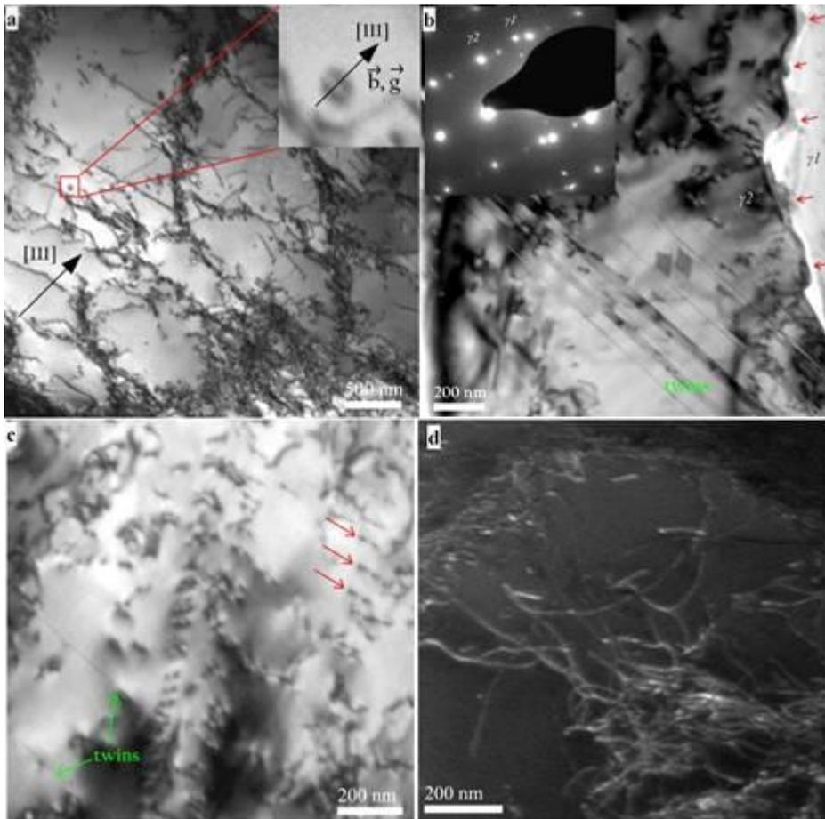
Fig. 1(a-d) Defect structures in SS 316LN subjected to LCF testing at 923K
