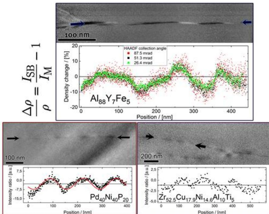
Fig.1. Alternating (periodic) high and low density regions in shear bands for different metallic glasses.
