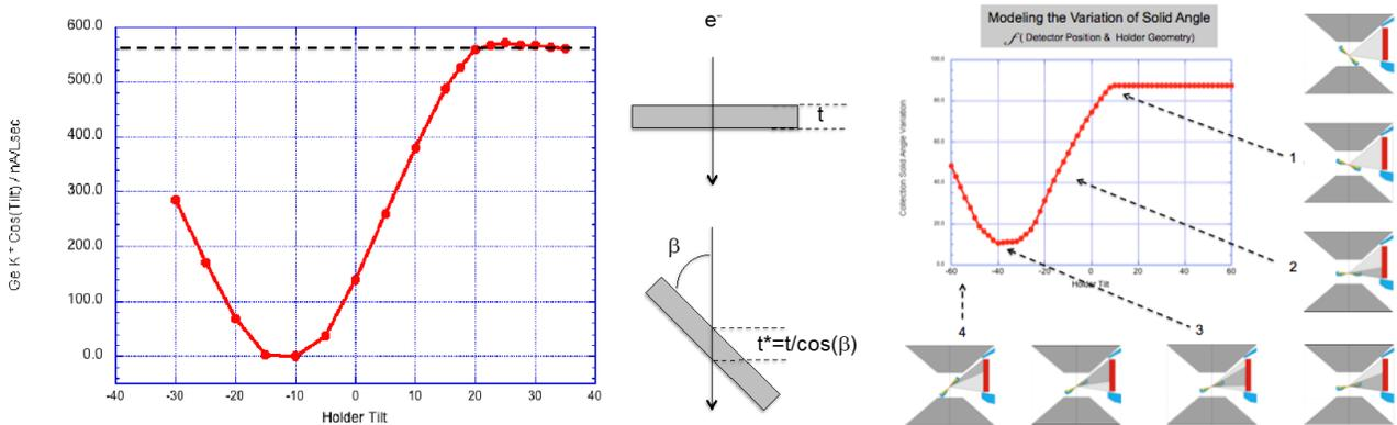
Figure 1. Experimental variation of the GeK with holder tilt. Vertical axis = Ge K integral \* Cos (tilt) /nA/LiveSec.
