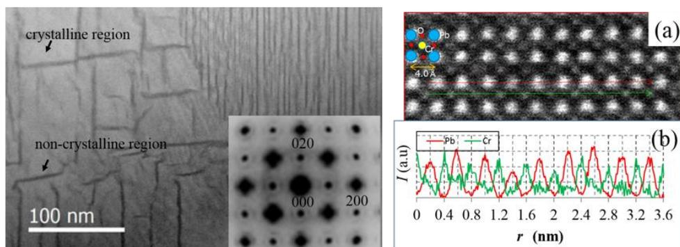
Fig. 1. (a) Atomic-resolved HAADF-STEM image showing the coexistence of the crystalline and non-crystalline phases. (inset) Electron diffraction pattern obtained from the coexisting region. Halo-pattern and diffuse scatterings can be clearly seen.
