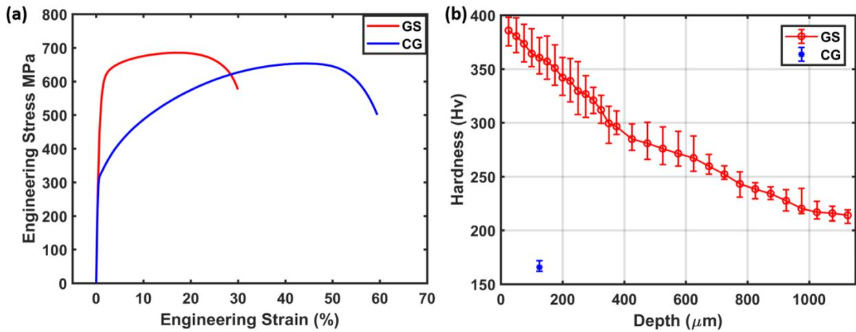
Fig.1: (a) Engineering Stress - Strain curves and (b) Hardness of a CG sample and of a sample with GS.
