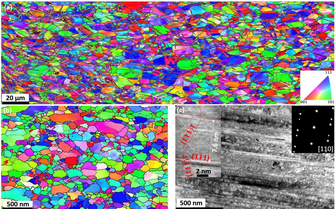
Fig.2: (a) An EBSD map from the surface to a depth of 250  $\mu\text{m}$ , (b) a TKD map at the top surface area, and (c) a TEM image taken from an area  $\sim 20 \mu\text{m}$  from the surface, showing a high density of twins. Insets on the upper left and right corner of (c) are a high-resolution TEM image and an electron diffraction pattern, respectively, evidencing the existing of twinned structures.
