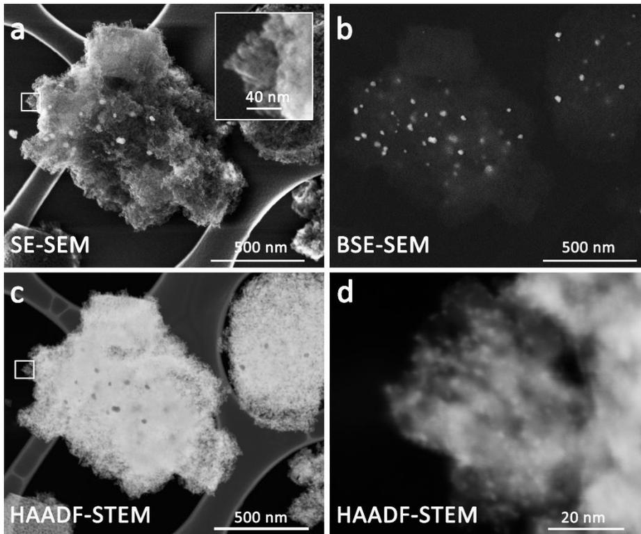
Figure 1. Pt nanoparticles on a porous  $\text{Al}_2\text{O}_3$  carrier imaged at 30 keV by a) SE-SEM, b) in-lens BSE-SEM, c,d) overview and high-magnification HAADF-STEM.
