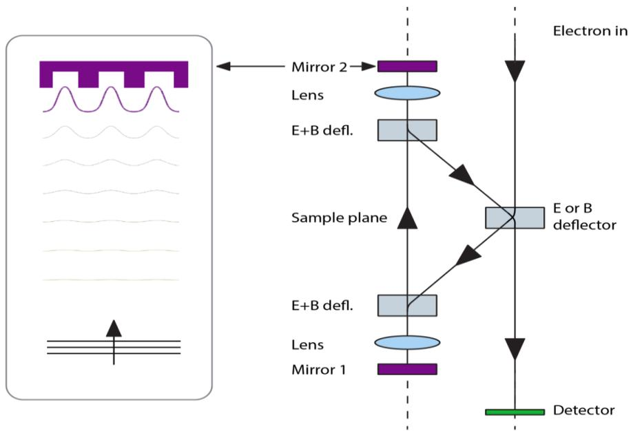
Figure 1. (left) Modulation of the mirror potential as a result of a grating-like pattern. The incident plane electron wave experiences path length differences upon reflection. This modulates the phase and is expected to result in diffraction spots when imaged towards a sample plane. (right) Schematic of the mirror setup placed inside the sample chamber of an SEM.
