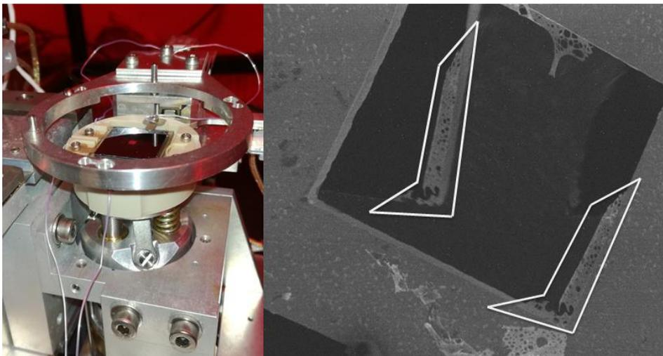
Figure 2. (left) The lens and mirror MEMS stack positioned on a translation and tilt stage for alignment. The sample holder is removed in this picture. (right) Micrograph of primary and mirror image in the same plane. The white shape indicates top and bottom of the same position on a sample. Full width 100 micrometer.
