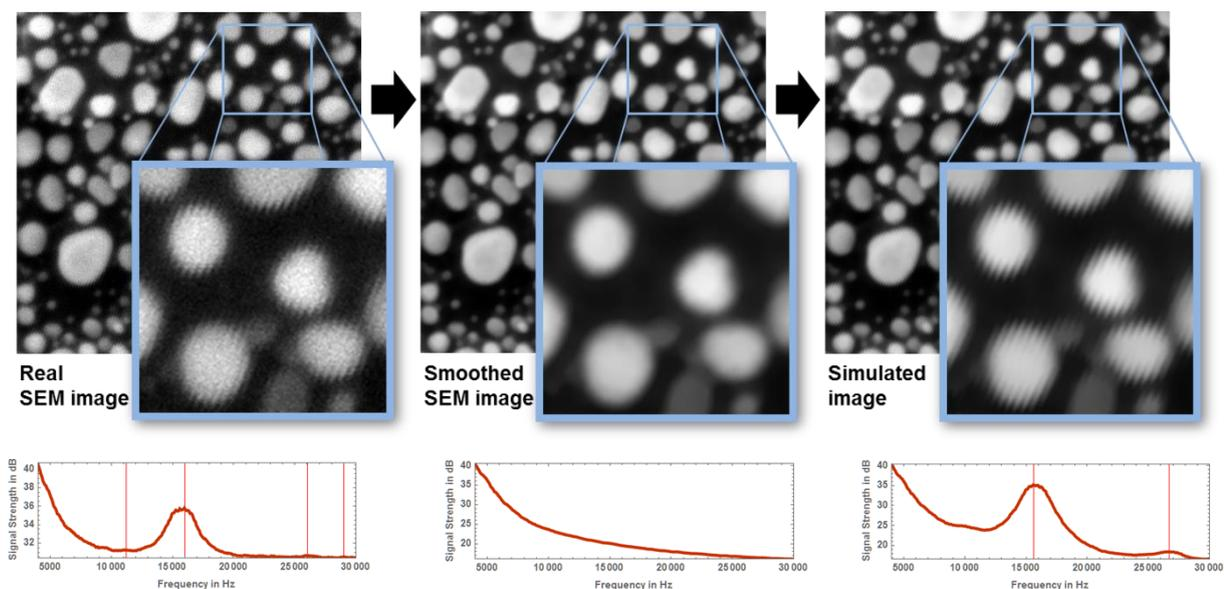
**Figure:** Top row: SEM image exhibiting high frequency noise artefacts (left). Numerically smoothed and sharpened image (centre) used for numerical simulation of electron beam dislocation-induced effects (right). Bottom row: Spectral analysis results of the real and synthetic images.
