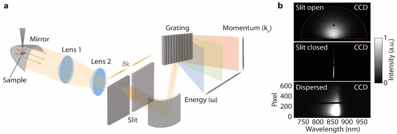
**Figure: (a)** Experimental realization of the E-k momentum imaging. **(b)** Images of a CL Fourier pattern from a GaAs crystal measured with slit open, slit closed and dispersed by the grating. The latter corresponds to a hybrid E-k image.
