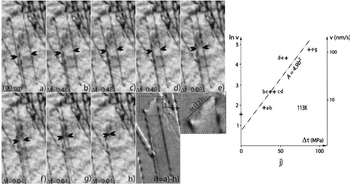
Fig. 2: Dipole annihilation at 113 K in pure iron. The velocity of two opposite screw dislocations increases as their distance decreases (note the decreasing time intervals  $Dt$  between two successive images). The increase in velocity as a function of the interaction stress  $Dt$  in (j) yields the microscopic activation area  $A$ .
