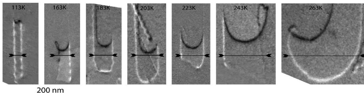
Fig. 1: Series of dipole expansions at increasing temperatures in pure iron. Note the increase of the critical distance arrowed, which corresponds to the decrease of the local stress with increasing temperature.
