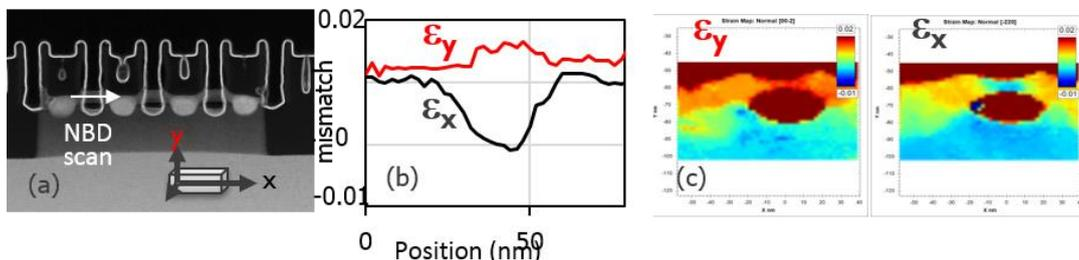
Figure 1 HAADF-STEM imaging (a) NBD strain profile (b) and mapping (c) on released wire
