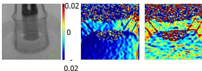
Figure 2 GPA [4] when germanium and tungsten overlap
