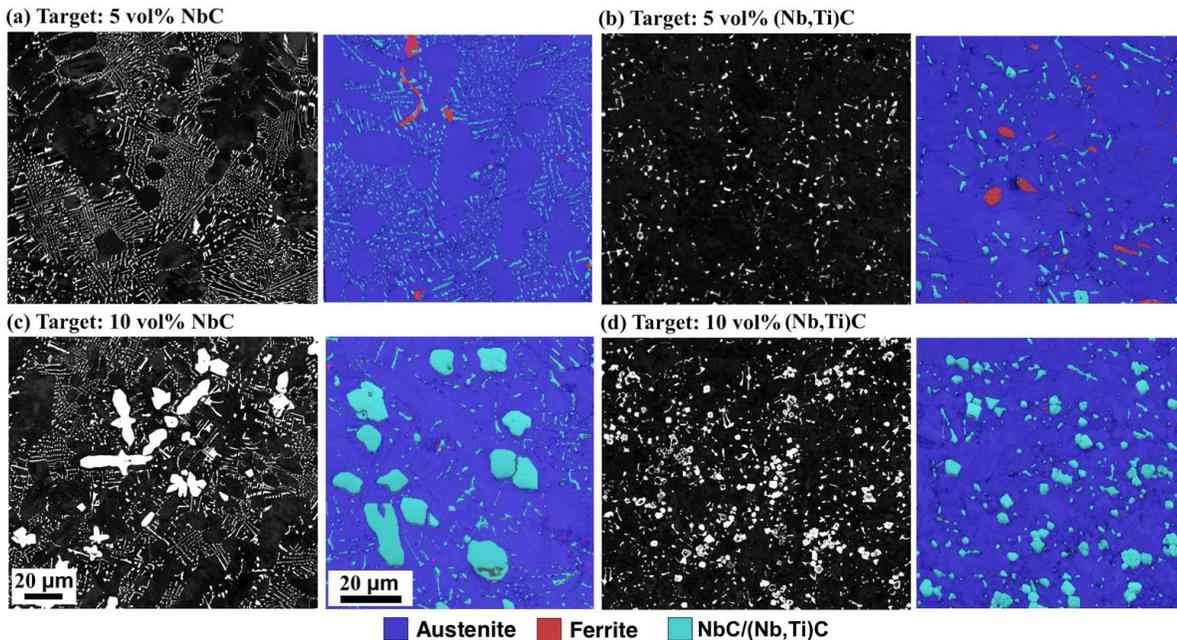
QBSD SEM images and EBSD phase maps showing the carbide morphology and phases present in austenitic stainless steels containing NbC or  $(\text{Nb}, \text{Ti})\text{C}$  [3].
