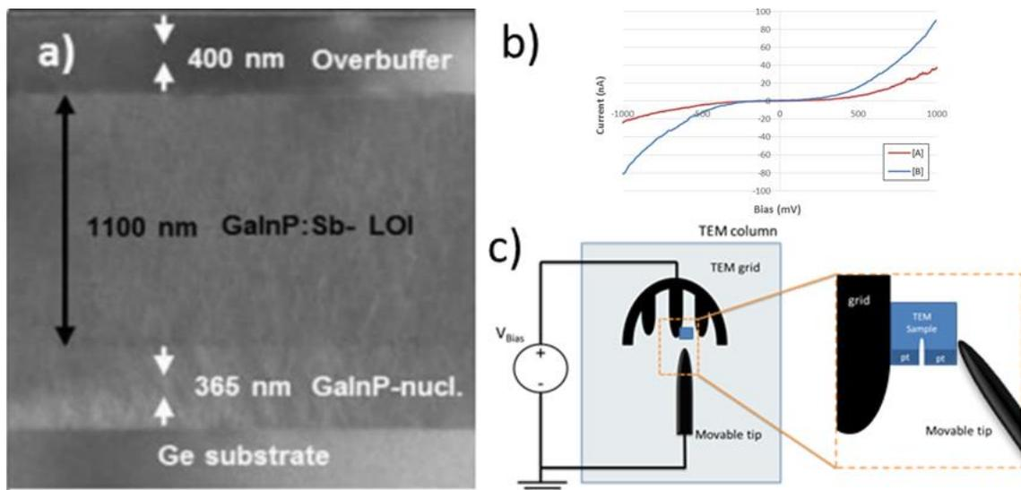
**Figure:** (a) low magnification TEM image of the sample, (b) I-V characteristic of the sample for the two orthogonal [110] and [1-10] directions, (c) schematic of the *in-situ* biasing in a TEM system.
