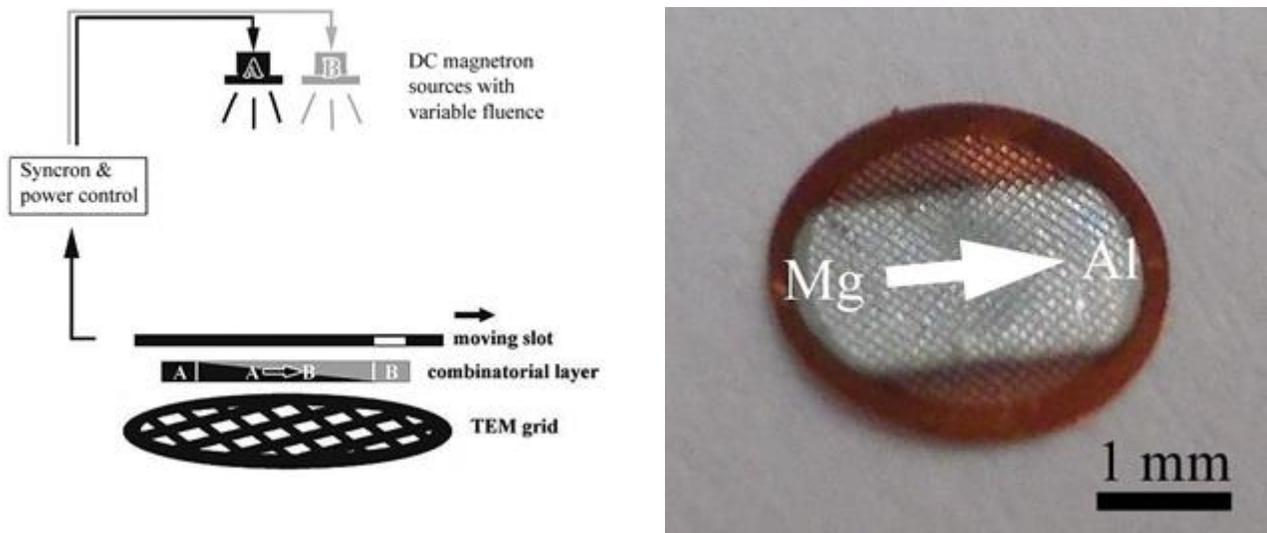
Figure 1. (a) Set-up of micro-combinatorial deposition for TEM samples. For nanoindentation the sample size is scaled up to 25mm. (b) Photo of a combinatorial Mg-Al sample on a 300-mesh TEM grid that exhibits a 1.5 mm long gradient section embedded between pure Al and Mg domains.
