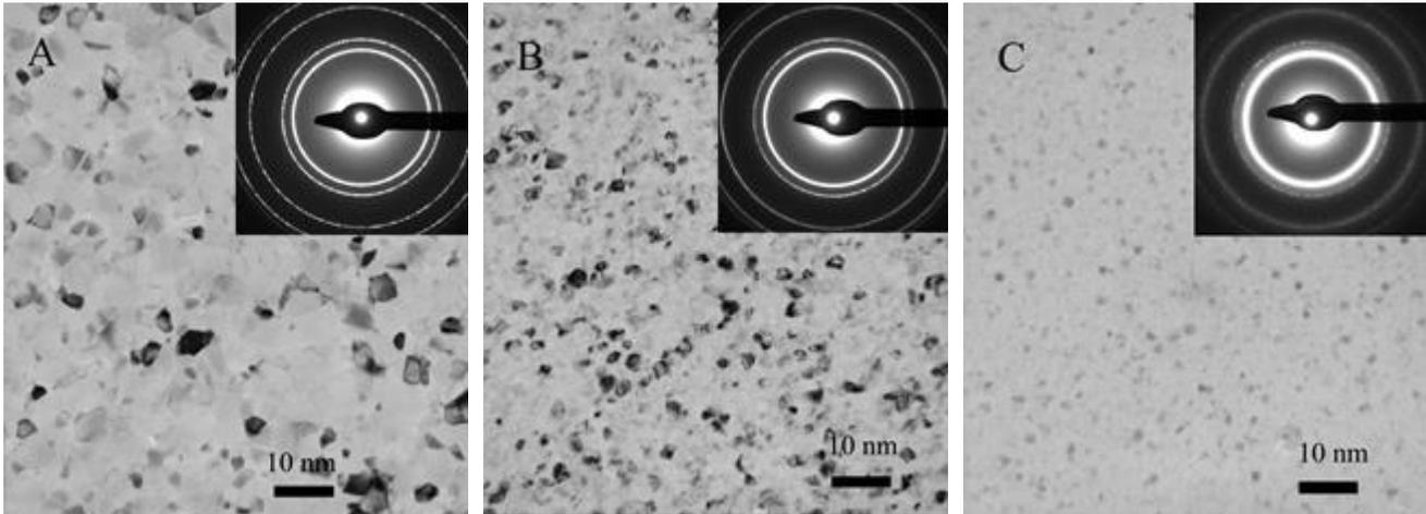
*Figure 2. BF TEM images with SAED insets of (a) 1%, (b) 10% and (c) 30% Mg/Al showing remarkably different grain size and structure revealed from a single  $\mu$ -combinatorial sample.*
