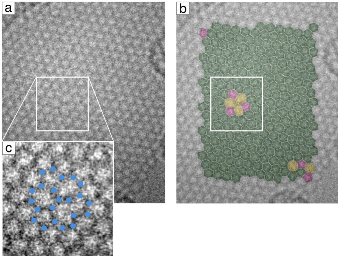
Figure 1. (a) Low-dose image of a graphene sheet recorded with a 50ms exposure at 80KV containing defects; (b) Automatically generated annotation with 5-membered rings (pink), 6-membered rings (green), and 7-membered rings (yellow) overlaid on top of the experimental image; (c) enlarged defect area with carbon atom positions marked by blue circles.
