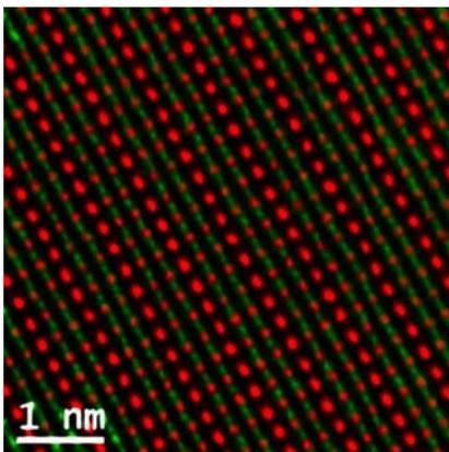
**Figure 2.** Spin-Orbit Kagome Metal,  $\text{Fe}_3\text{Sn}_2$ . High Angle Angular Dark Field Image (HAADF) overlaid with atomic number contrast false coloring (right).
