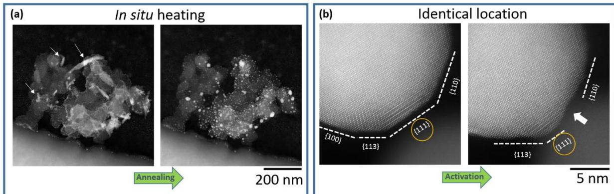
Fig.1. (a) Formation of  $\text{PtCu}_3$  nanoparticles during the *in situ* heating STEM experiment. Left, CuPt nanoparticles at room temperature with Cu needles (marked with arrows). In the right, CuPt nanoparticles after the annealing process at 500 °C and further 800 °C. (b) Neighboring facets of  $\{111\}$  get preferentially dealloyed, observed by identical location STEM after the activation protocol.
