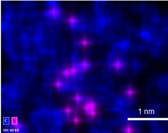
Figure 2: Single sulphur atom captured moving with the electron beam on carbonaceous material during a single scan. Single frame map acquired in 60 seconds using an oval 100mm<sup>2</sup> EDS detector with 0.7sr solid angle in a dedicated Cs-corrected cold FEG UHV STEM at 60kV. Sample and data courtesy: R. Stroud, NRL, Washington, USA [2].
