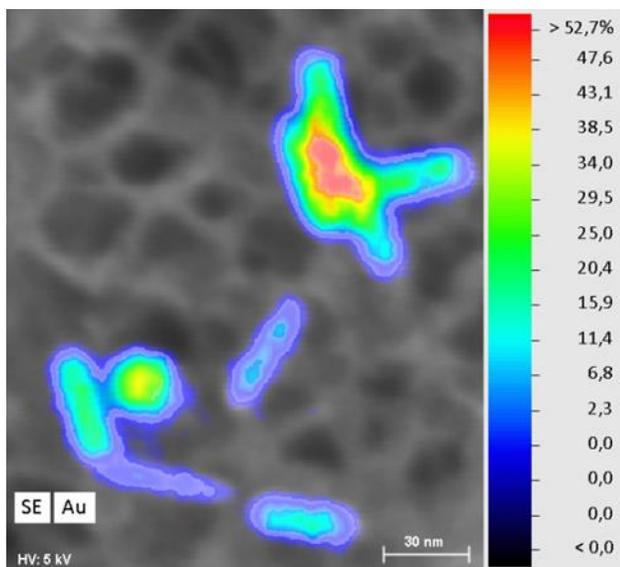
Figure.1: Gold nanoparticles on porous titanium oxide implant surfaces, used to lower the infection risk. They change the electric surface potential making it fatal for settling bacteria. High collection, high take-off angle low kV EDS in SEM helps to quickly judge the distribution and embedding of various nanoparticle types, sizes and shapes on the porous oxide surface of the potential implant. These data can be correlated with light microscopy
