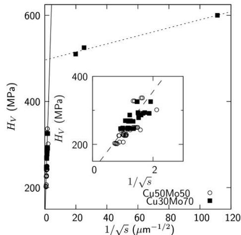
Figure 2: Hall-Petch plot showing the hardness of Cu-Mo composites versus the inverse square-root of the lamellar spacing,  $s$ .
