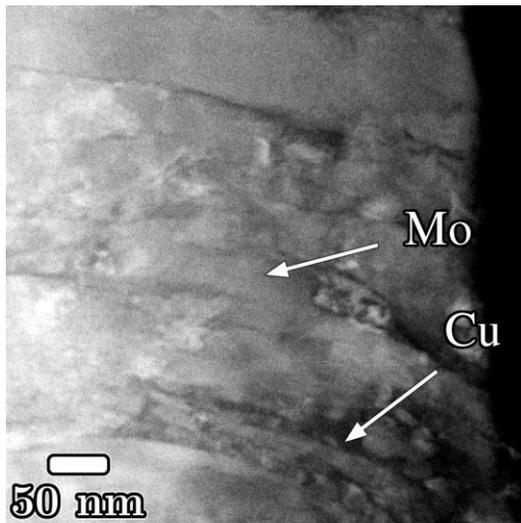
Figure 2-: HAADF-STEM micrograph showing the microstructure of a Cu<sub>30</sub>Mo<sub>70</sub> (wt.%) composite. Cu and Mo lamellae vary in thickness and orientation. The shear direction is in the horizontal plane.
