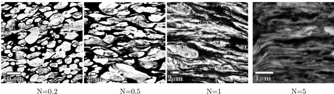
Figure 1: Backscattered scanning electron micrographs showing the microstructure of a Cu<sub>30</sub>Mo<sub>70</sub> (wt.%) composite with increasing number of rotations of HPT deformations, N.
