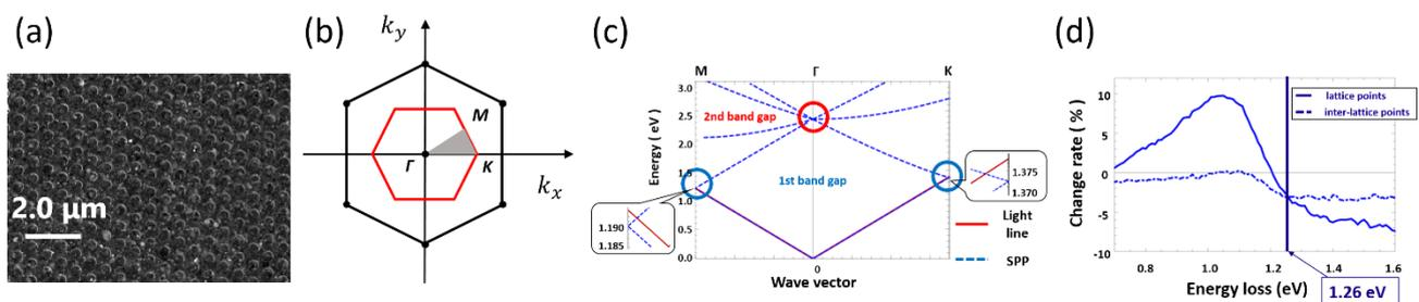
Fig. 1 (a) A STEM image of the Tri-PIC film, (b) a reciprocal lattice of the triangular lattice, (c) the plasmonic band structure of the Tri-PIC under the empty lattice approximation, (d) Change rates extracted from the lattice points and the inter-lattice points.
