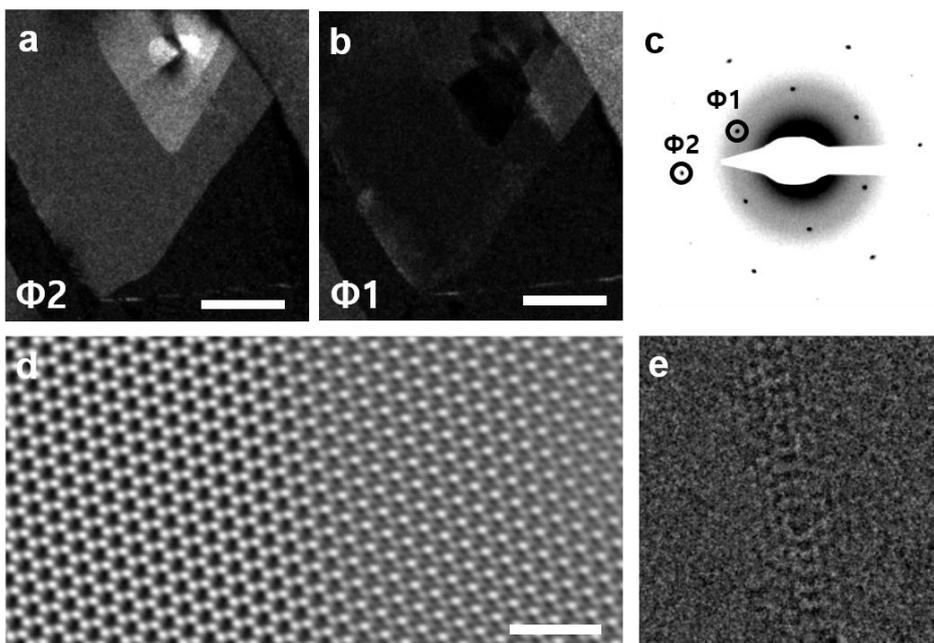
Figure 1. Atomically thin twin boundary in AA'- and AB-stacked hBN film. (a,b) Dark field TEM images of triangular, few-layer hBN islands from a second-order diffraction spot ( $\Phi_2$ ), and a first-order diffraction spot ( $\Phi_1$ ) displayed in (c). (d), HR-TEM image of the stacking boundary of a tri-layer ABA/AA'A-stacked hBN film.
