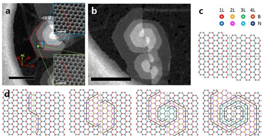
Figure 1. Double helical structure of few-layer hBN islands. (a) DF-TEM and HR-TEM image in few-layer a hBN island. (b) Double helix divided by domain boundary in DF-TEM image. (c) Atomic model of aligned hBN domain boundary. (d) Growth mechanism of hBN spirals. Scale bar in (a,b), 0.2 $\mu$ m and (a) inset, 1nm.
