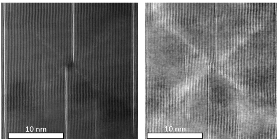
Figure 2. Simultaneously acquired ADF (left) and ABF (right) STEM images showing the resulting cross-shaped lattice strain from the adjacent termination of two monolayers
