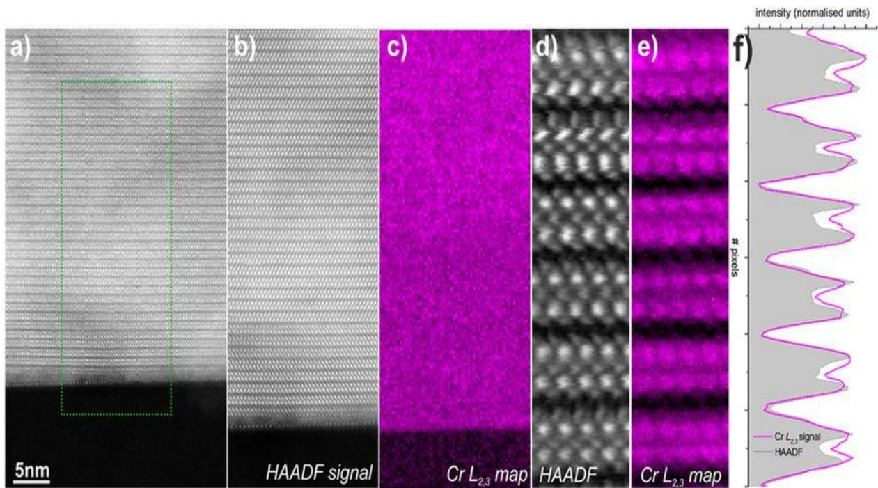
Fig. 2. **(a)** HAADF-STEM survey of Bi<sub>2</sub>Se<sub>3</sub>/Al<sub>2</sub>O<sub>3</sub>. **(b)** HAADF-STEM from the region of interest. Acquired simultaneously with the Cr L<sub>2,3</sub> EELS signal **(c)** showing uniform distribution of Cr. **(d)** Atomically resolved HAADF-STEM image from the film area recorded simultaneously with the EELS signal shown in **(e)**. **(e)** Cr L<sub>2,3</sub> EELS showing substituting of Bi.
