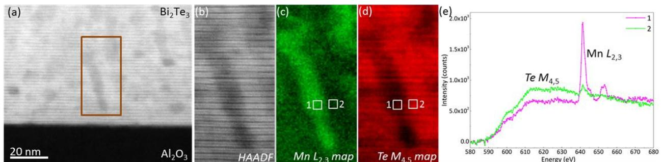
Fig.1 (a) HAADF-STEM survey image from the  $\text{Bi}_2\text{Te}_3$ . (b) HAADF-STEM from the region of in (a) acquired simultaneously with the Mn  $L_{2,3}$  EELS signal (c) showing a higher concentration of Mn in the dark feature observed in the image. (d) The Te  $M_{4,5}$  EELS signal shows a distribution anti-correlated to that of Mn. (e) Mn  $L_{2,3}$  and Te  $M_{4,5}$  edges obtained from the grain-boundary and off-boundary regions labelled as 1 and 2 in (c) and (d).
