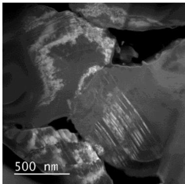
Figure 2. ADF-STEM image of diamond-diamond contact points formed in a binderless sample.
