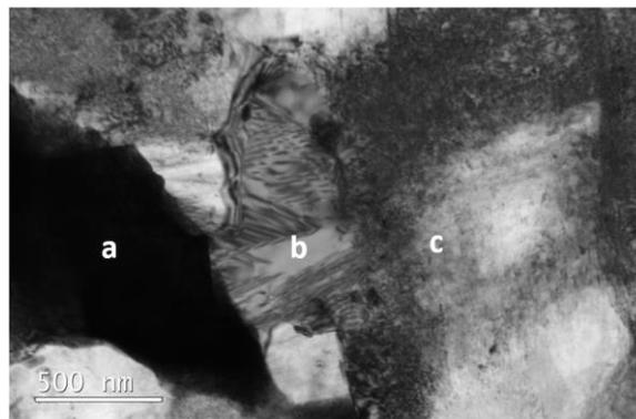
Figure 3. BF-TEM image of the infiltration sample showing: (a) residual cobalt metal pool, (b) reprecipitated diamond and (c) plastically deformed diamond.
