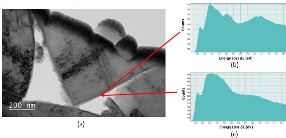
Fig.1. (a) BF image of binderless PCD with (b) graphite and (c) amorphous carbon EELS spectra.
