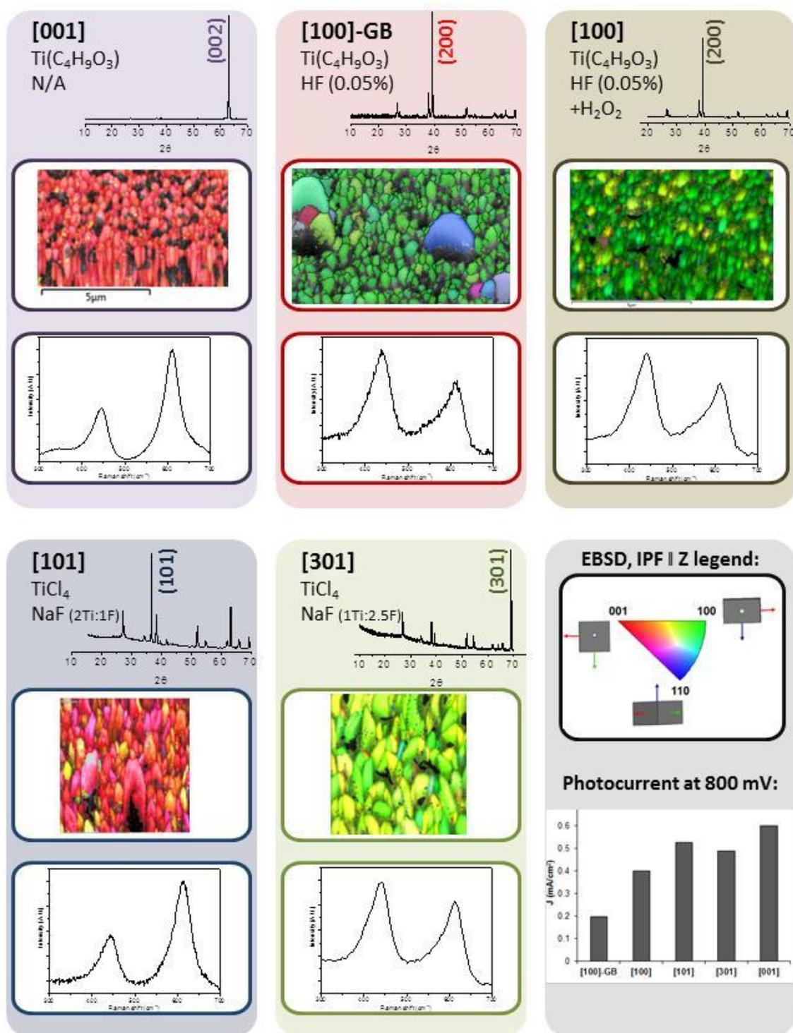
Figure 1. Characterization of rutile TiO<sub>2</sub> photoanodes for water splittings with different crystal orientations: X-ray diffractogram, Orientation map (IPF Z), raman spectra and their photoelectrochemical efficiency determined as the photocurrent measured at 800mV vs Ag/AgCl (3M).
