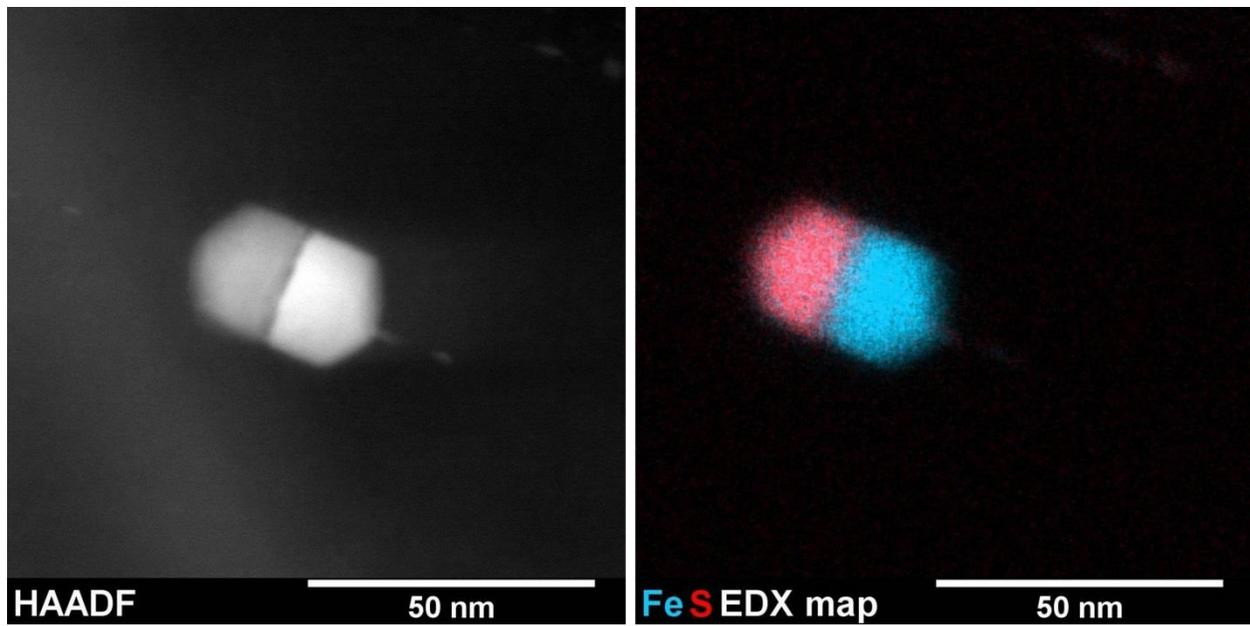
Figure 1- HAADF image and EDX map of an Fe-S type inclusion in diamond matrix.
