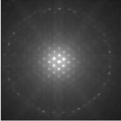
**Figure 1:** Diffraction pattern from Silicon substrate of a 14 nm semiconductor device at  $[100]$  zone axis taken at 30 kV.
