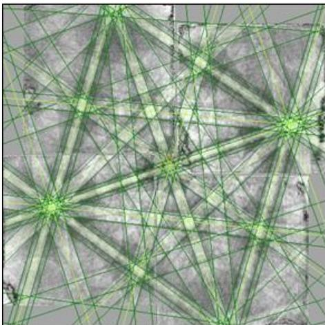
**Figure 3:** Acquired and automatically indexed EBSD of monocrystalline iron (ferrite) in tilt-free geometry.
