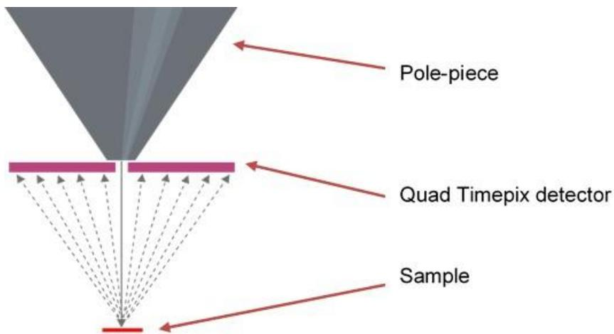
**Figure 2:** Setup of EBSD tilt-free method. Detector is placed directly below pole-piece with sample parallel to the detector.
