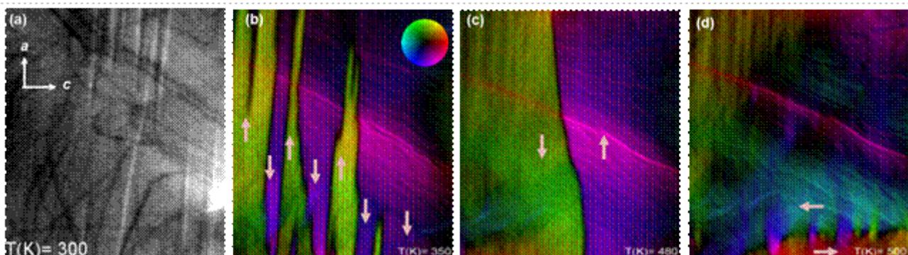
Figure 2. (a-c) Magnetic structure transition under magnetic field that were applied normal to sample plane at 530 K. (a) Helical stripe structure in the zero magnetic field. (c) Biskyrmion spin texture formed by applying magnetic field of 0.1 T. (d) Enlarged diagram of the biskyrmion crystal. Colors and arrows show the direction of electron spin in the biskyrmion.
