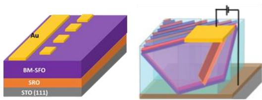
Figure 1 Resistive switching memory device with  $\text{Sr}_2\text{Fe}_2\text{O}_5$
