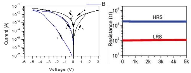
Figure 2 Measurements of I-V curve & resistance
