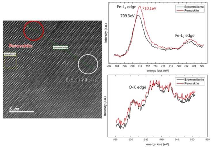
Figure 4 HAADF STEM image and EELS data between Perovskite and Brownmillerite structure.
