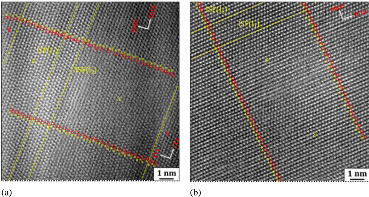
Fig. 2 HAADF STEM micrographs showing  $\epsilon$ -ISFs of type  $I_2$  and  $I_1$  after plane strain compression/cold-rolling to (a) 15% and (b) 42% thickness reduction. Zone axes are  $[110]_{\gamma}$ ,  $[\bar{1}2\bar{1}0]_{\epsilon}$  in Fig. 2a and  $[\bar{1}2\bar{1}0]_{\epsilon}$  in Fig. 2b.
