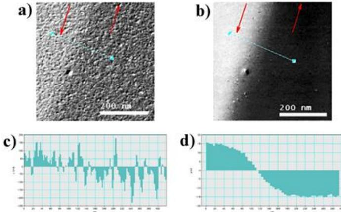
Fig. 1: Comparison of magnetic imaging of domain wall in 20 nm thick Permalloy, a) segmented detection b) pixelated detection, c) single line profile of domain wall (segmented detection), d) same profile (pixelated detection). Integrated magnetic induction orientation is shown by red arrows. Probe convergence semi-angle was 0.537mrad and camera length was 3 m.
