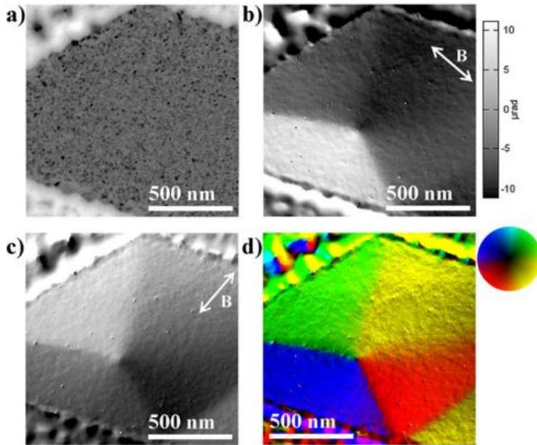
Fig. 2: Medipix3 imaging of patterned 20 nm thick Permalloy in which a magnetic vortex was formed. (a) is a bright field image reconstructed by sum of CBED disk, (b) and (c) are two orthogonal components of integrated magnetic induction, orientation is shown by double-headed arrows, (d) a colour image showing the orientation and magnitude of the induction. Probe convergence semi-angle was 2.15mrad and camera length was 6 m.
