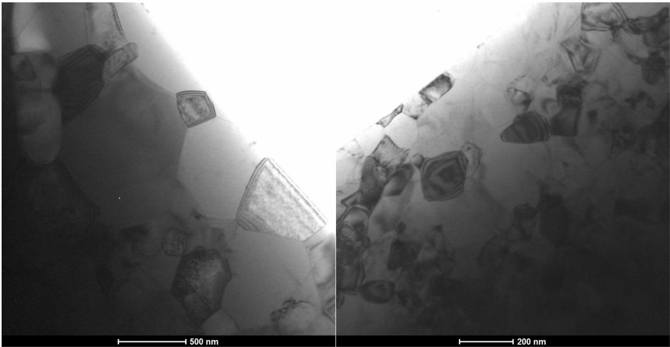
Figure 2 Two Bright Filed TEM images from microwire specimens prepared by the introduced method.
