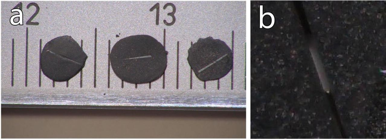
Figure 1 (a) Ni-Ti microwire embedded in resin and grinded to 80µm thickness; (b) Electropolished microwire with hole in the center of the microwire.
