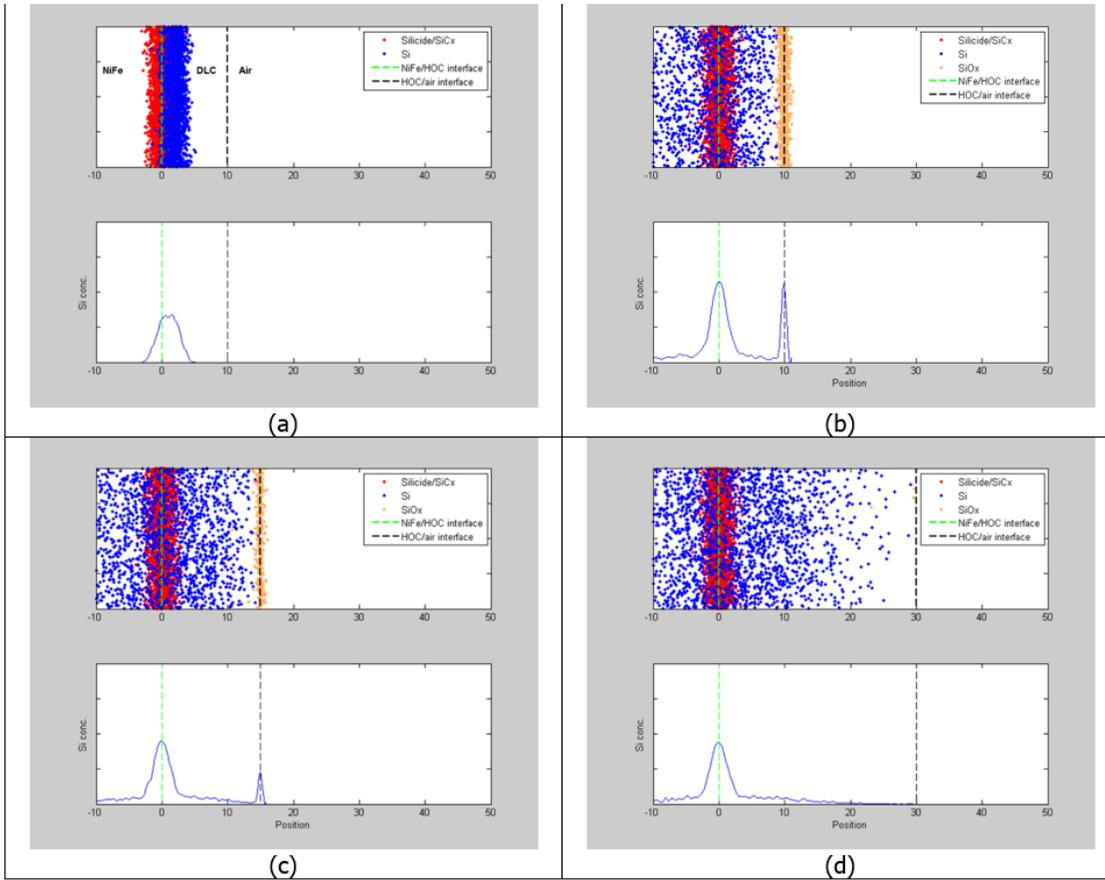
Figure 01 - Random-walk Monte Carlo simulation of the Si diffusion effect. As-deposited film stack on a 10 Å DLC film is shown in (a). After Si diffusion, the end-states are shown for DLC: (b) 10 Å, (c) 15 Å and (d) 50 Å. The acronym HOC refers to head overcoat, or the totality of seed layer plus DLC protective system.
