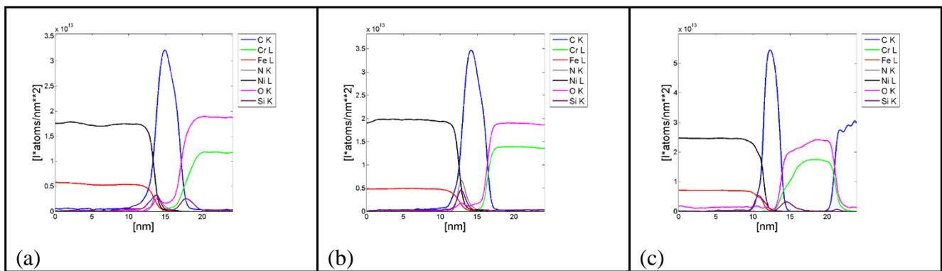
Figure 02 - EELS elemental profiles showing three types of Si-containing seed were studied: sub-stoichiometric Si<sub>x</sub>N<sub>y</sub> with N/Si = 0.44 (a), stoichiometric Si<sub>3</sub>N<sub>4</sub> with N/Si = 1.33 (b), and Si-only seed (c).
