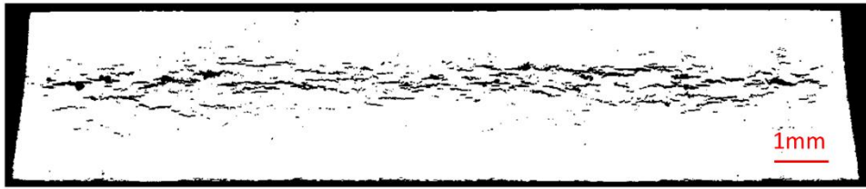
Fig.(1) Processed optical image of the recovered sample of LDX2101 form plate impact experiment at an impact velocity of 264 m/s.
