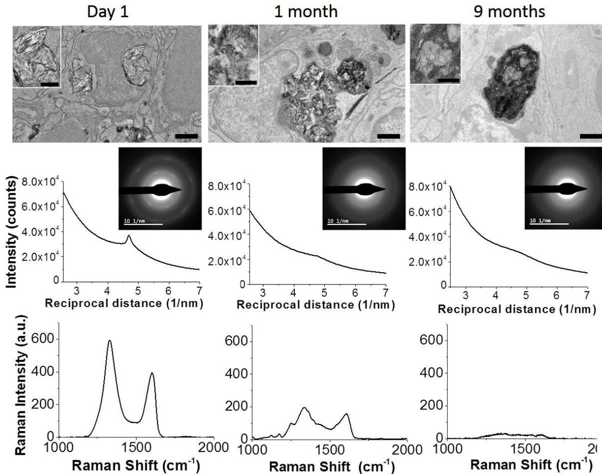
Figure 1. First row: TEM images of spleen tissue for 1 day, 1 month and 9 months (scale bars 1 μm and 0.5 μm in the insets); second row: corresponding electron diffraction patterns (inset) and line profiles demonstrating the identification of GO at the ultrastructural level; third row: corresponding Raman spectra (D and G peaks) showing the degradation of GO over time.
