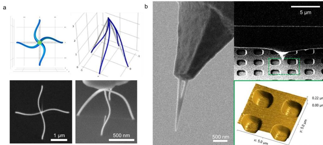
**Figure 2 Iterative adoption of our model to optimize the functionality. (a)** by adopting our FES model, we unravel the underlying mechanical properties of these structures. **(b)** finally, we deploy optimized Pt based 3D nanoprobes on AFM cantilevers to demonstrate their imaging capability.
