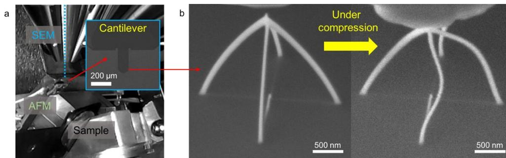
**Figure 1 Correlative *in-situ* force measurements.** **a**, the combined AFM - SEM measurement setup. **b**, utilizing the combined approach, even nanoscale structures can be directly accessed and with a prepared cantilever the dynamic behavior of such structures can be studied under force load.
