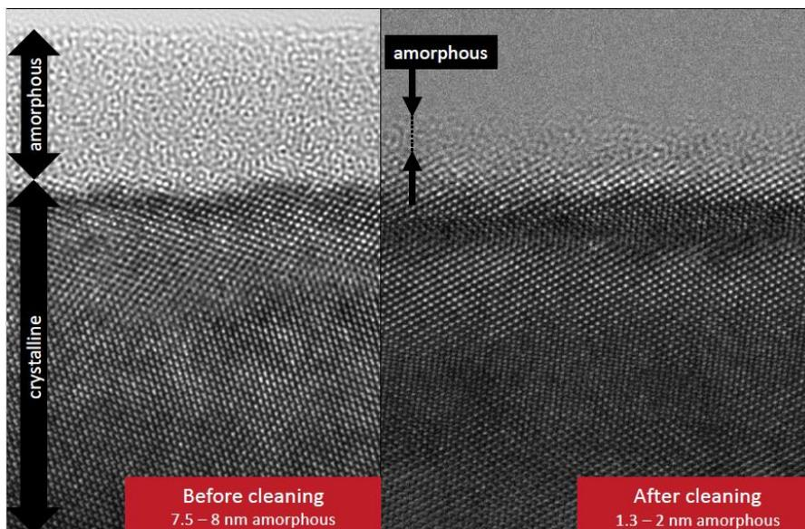
Figure 1: HRTEM images of a Si lamella prepared by Ga FIB before and after cleaning with uPolisher showing the reduction in the amorphous layer at the edge from ~8 nm to 2 nm.
