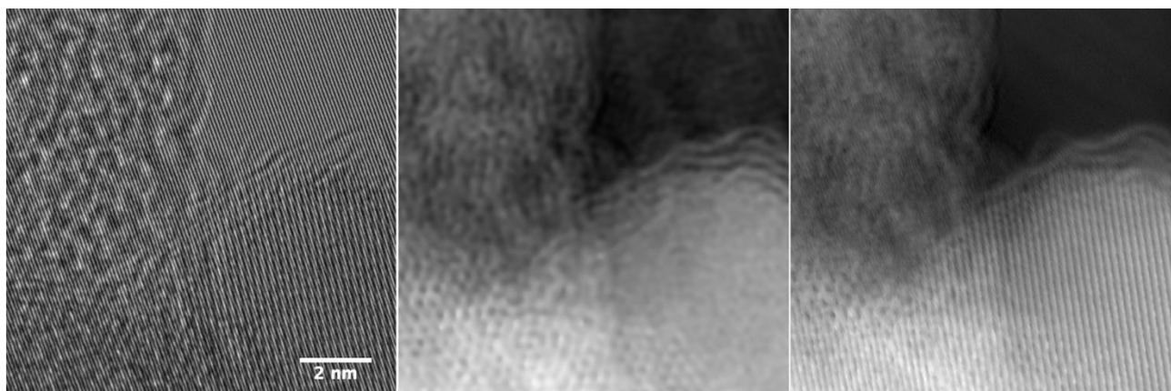
Figure 1. (a) Single hologram of CeO<sub>2</sub> on a carbon film. (b) Exit wave phase reconstructed by the conventional Fourier method. (c) Exit wave phase iteratively reconstructed from a series of 26 phase-shifting holograms.
