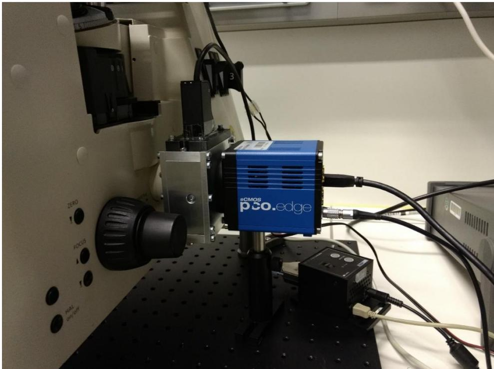
Image 2: The add-on camera module PIAH attached to a standard optical microscope. It allows to image cell quantitatively without staining.
